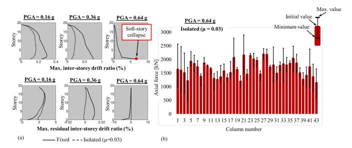
Figure 6. (a) peak global responses resulted from nonlinear response history analysis at three Peak Ground Accelerations, (b) average value of first floor columns' axial load variations for the isolated structure
