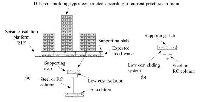
Figure 1. Resilient Seismic isolation platform (SIP) concept built to support buildings: (a) overview, (b) alternative low-cost isolation systems
