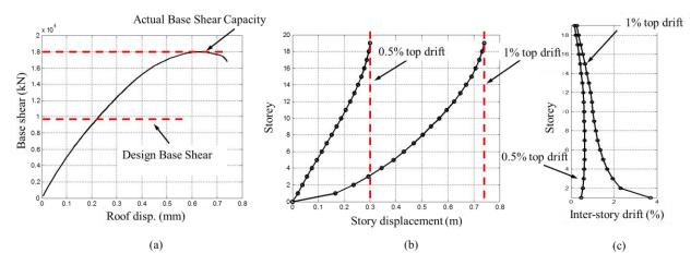
*Figure 3.Pushover analysis results: (a) base shear vs. roof displacement, (b) storey displacement, (c) inter-storey drift ratio* **Nonlinear response history analysis results with variable friction properties**
